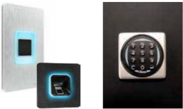
Biometric readers mounted on the door leaf and wall ISEO keypad installed on the door leaf, enabling opening via RFID and cards
