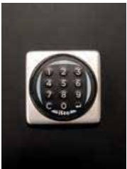
ISEO keypad installed on the door leaf, enabling opening via RFID and cards
